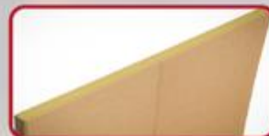
A50 Panel Fire classification A-15 Thickness 50 mm Acoustic attenuation 48db
